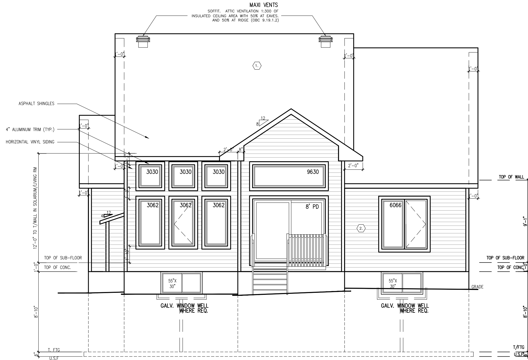
ELEVATION B SUN ROOM REAR ELEVATION
