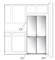
To ensure proper ventilation for your refrigerator, allow for a 1/2" (12.7 mm) space on each side and at the top. Allow for a 2" (50 mm) space behind the refrigerator. If your refrigerator has an ice maker, allow extra space at the back for the water line connections. When installing your refrigerator next to a fixed wall, leave a 3¾" (95 mm) minimum space between the refrigerator and wall to allow the door to swing open.
