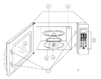
Door Safety Lock System Oven Window Roller Ring
