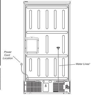
\*Water lines are not foamed in and are external.
