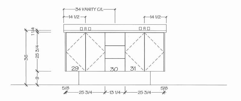
\*NOTE MEASURES ARE BASED ON FINISHED DRYWALL\*
