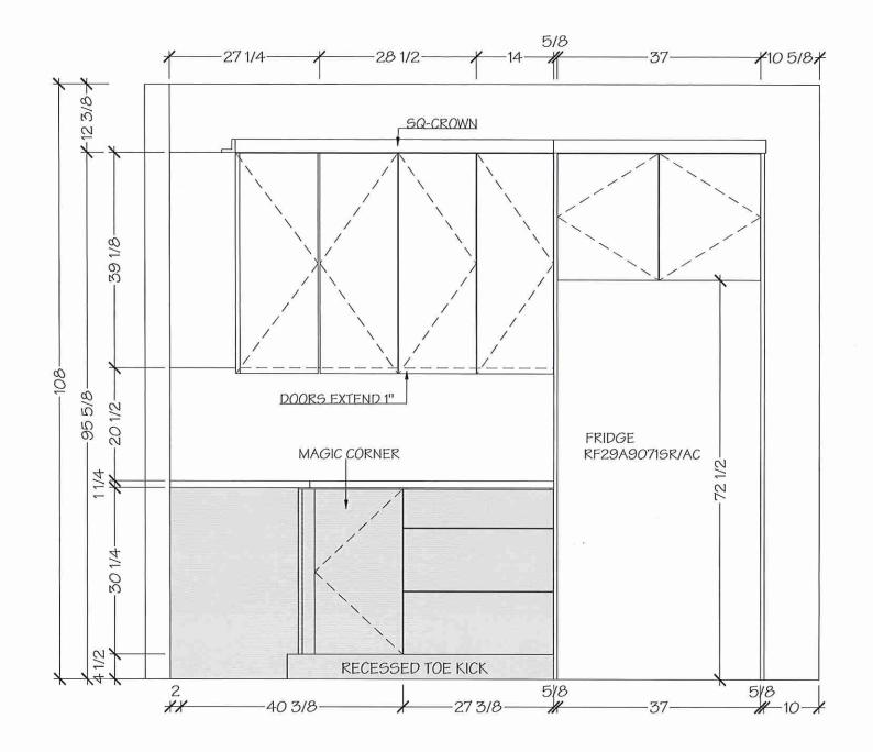
\*NOTE MEASURES ARE BASED ON FINISHED DRYWALL\*
