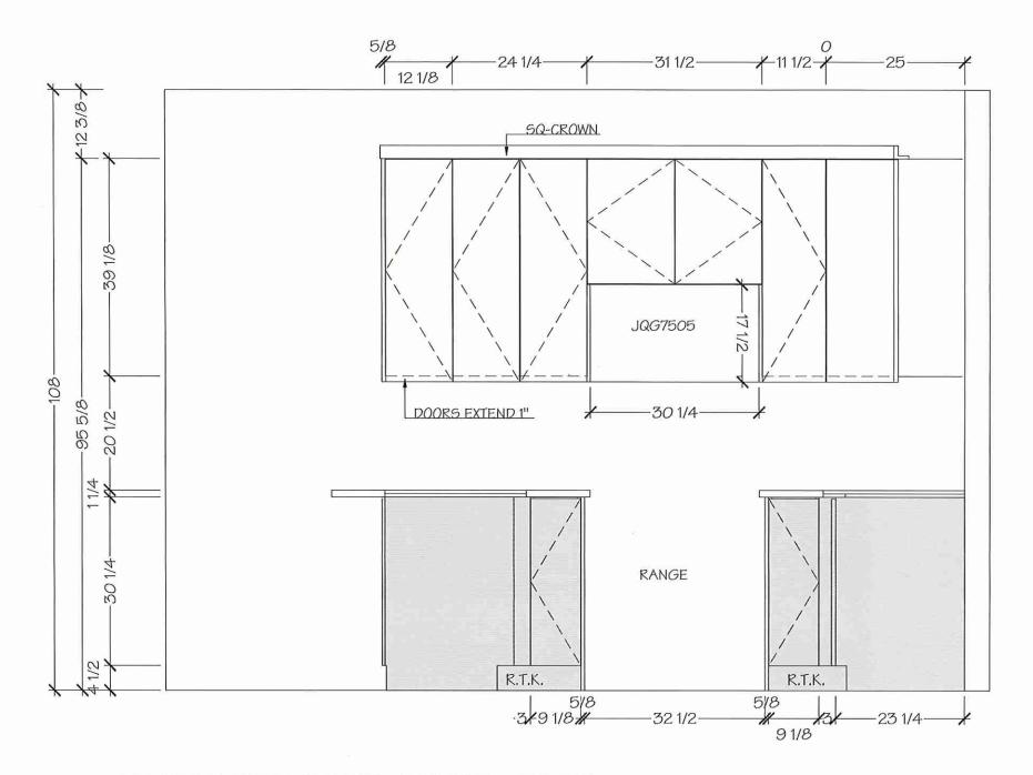
\*NOTE MEASURES ARE BASED ON FINISHED DRYWALL\*
