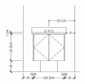
\*NOTE MEASURES ARE BASED ON FINISHED DRYWALL\*
