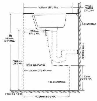
NOTE: \* Starred measurements comply with CSA B651 and OBC barrier free accessibility requirements.
