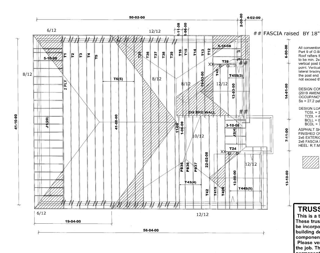
All conventional framing to conform with Part 9 of O.B.C. 2012 (2019 amendment). Roof rafters that cross over or meet trusses to be min. 2x4 SPF #2 @ 24" o/c with a vertical post to the truss at each cross point. Vertical posts longer than 6' to have lateral bracing so that the distance between the post end points and lateral bracing does not exceed 6'.
