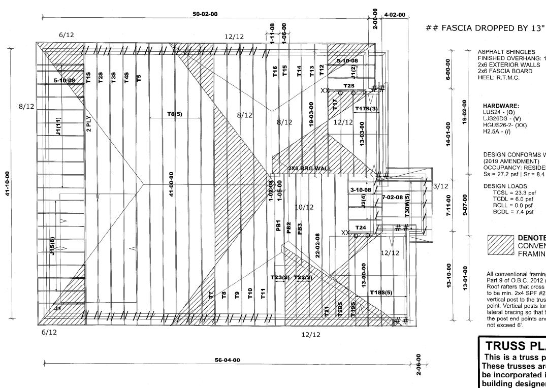
ASPHALT SHINGLES FINISHED OVERHANG: 12" 2x6 EXTERIOR WALLS 2x6 FASCIA BOARD HEEL: R.T.M.C.
