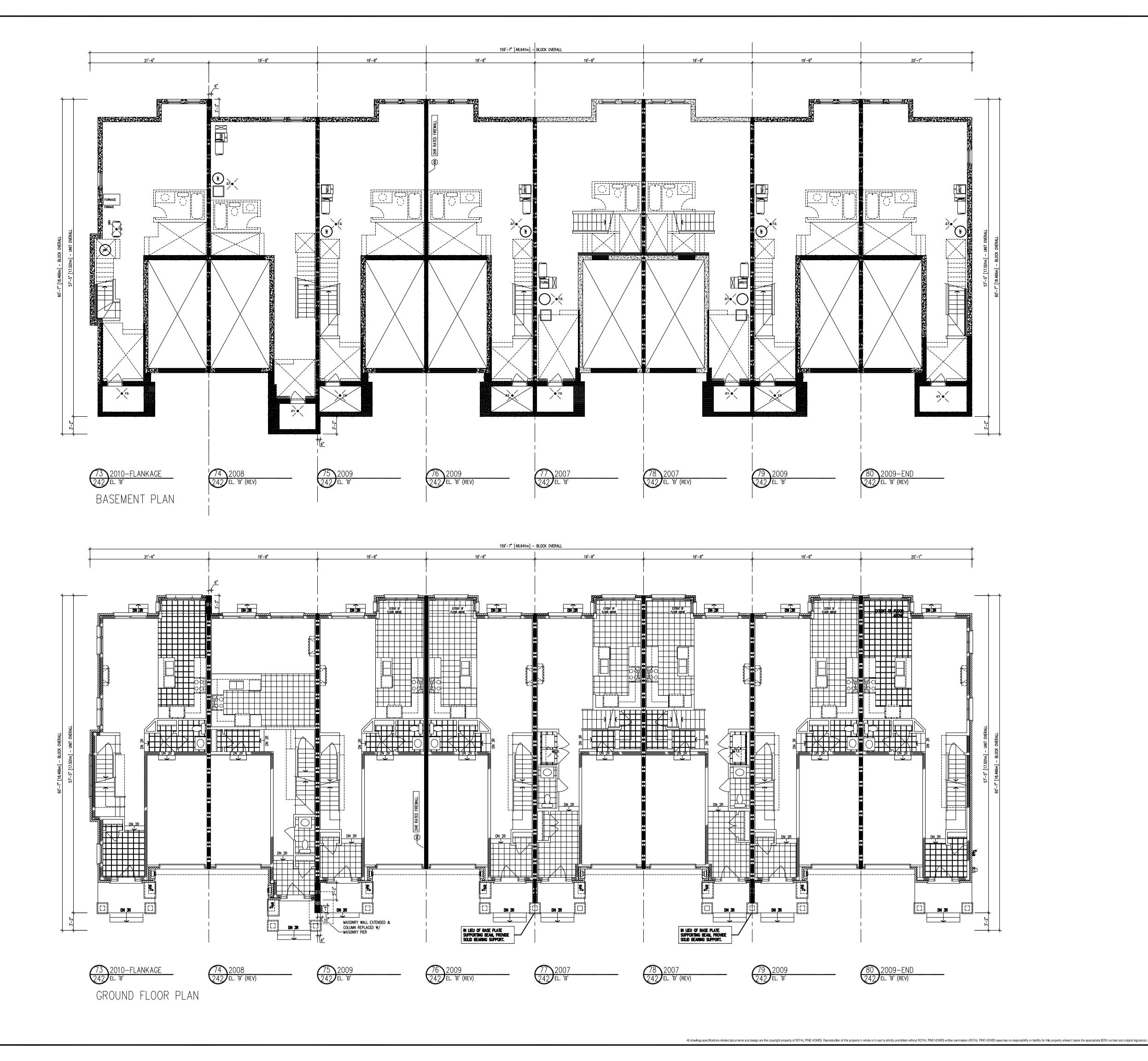
A FIREWALL IS REQUIRED IF THE BUILDING AREA IS GREATER THAN 600 m2 (6458 sq ft) AS PER BUILDING CODE PART 9 LIMITATIONS SECTION 1.1.2.4.(1) \*\* DEFINITION OF BUILDING AREA AS PER PART 1.4.1.2 IS THE EXTENT OF THE GREATEST HORIZONTAL BUILDING EXTERIOR WALLS ABOVE GRADE TO IF REQ'D THE CENTER OF THE FIREWALL (DEMISING LINE) BUILDING AREA CALCULATION FOR FIREWALLS AS PER O.B.C. PART 1 SECTION 1.1.2.4.(1). PART 3.1. & 9.10.
