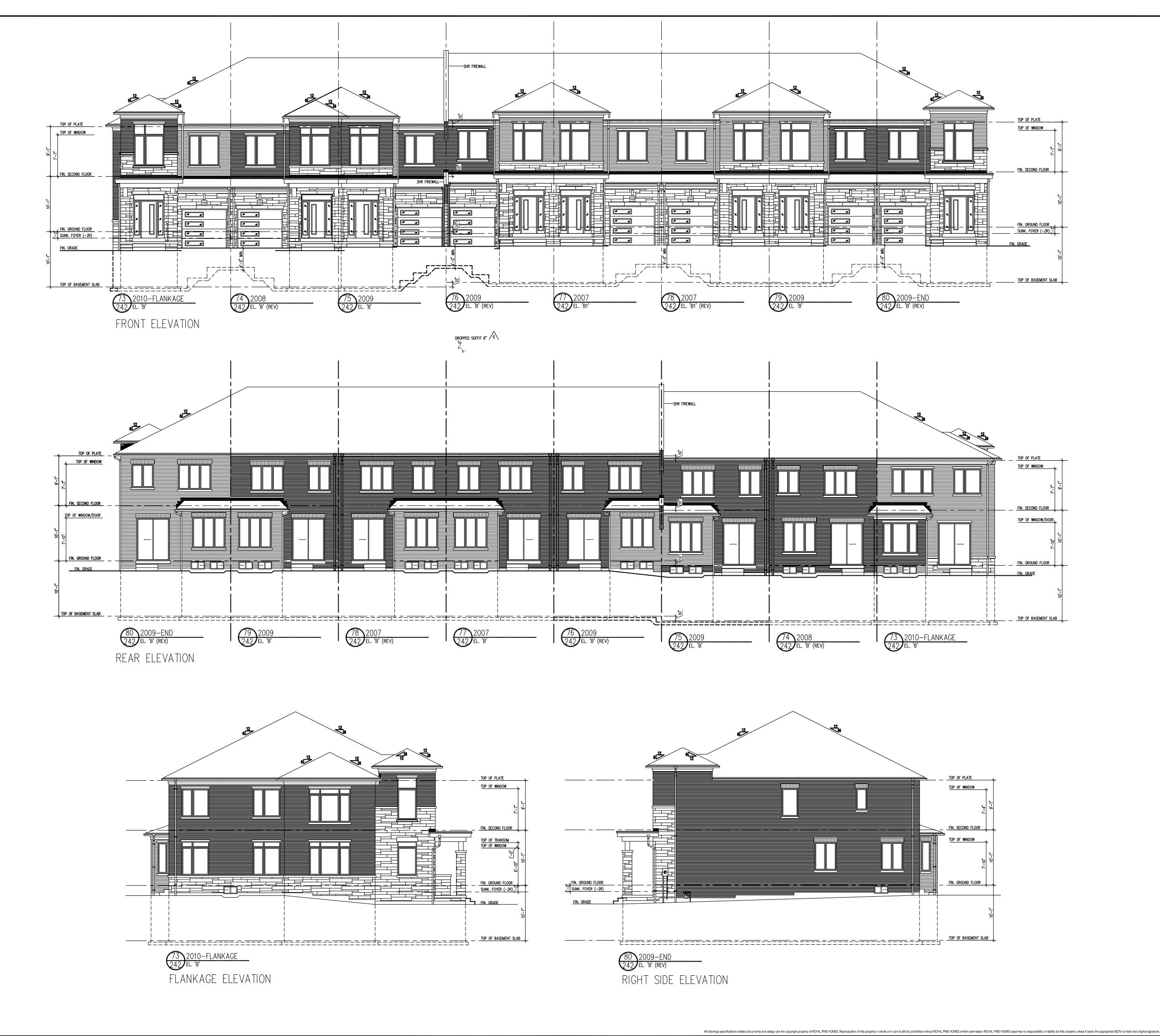
A FIREWALL IS REQUIRED IF THE BUILDING AREA IS GREATER THAN 600 m2 (6458 sq ft) AS PER BUILDING CODE PART 9 LIMITATIONS SECTION 1.1.2.4.(1) \*\* DEFINITION OF BUILDING AREA AS PER PÀRT 1.4.1.2 IS THE EXTENT OF THE GREATEST HORIZONTAL BUILDING EXTERIOR WALLS ABOVE GRADE TO IF REQ'I THE CENTER OF THE FIREWALL (DEMISING LINE) BUILDING AREA CALCULATION FOR FIREWALLS AS PE O.B.C. PART 1 SECTION 1.1.2.4.(1), PART 3.1. & 9.10.
