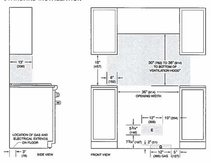
"Without ventilation hood, 42" (1087) minimum clearance countertop to combustible materials, charbroller and GR488 require non-combustible materials.
