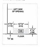
PANEL SPECIFICATIONS For complete panels specifications including width/height, weight requirements and thickness requirements visit <u>subzero-wolf.com/reveal</u>.
