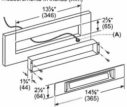
A: DBus Cable length: 30 feet (9180 mm)
