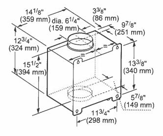
measurements in inches and mm
