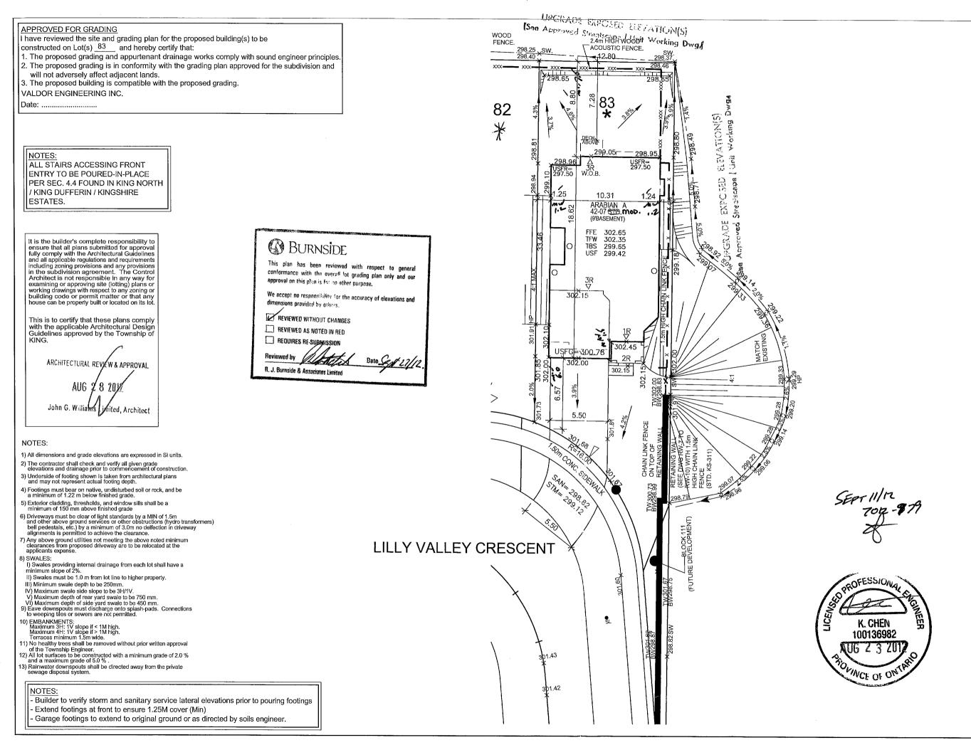
NOTE: BUILDER TO VERIFY LOCATION OF ALL HYDRANTS, STREET LIGHTS, TRANSFORMERS AND OTHER SERVICES. IF MIN. DIMENSIONS ARE NOT MAINTAINED BUILDER IS TO RELOCATE AT
