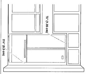
To ensure proper ventilation for your refrigerator, allow for a  $\frac{1}{2}$ " (1.25 cm) space on each side and at the top. Allow for 1" (2.54 cm) of space behind the refrigerator. If your refrigerator has an ice maker, make sure you leave some extra space at the back for the water line connections.
