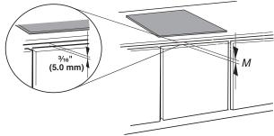
**NOTES:** After you make the countertop cutout, some installations may require notching down the base cabinet side walls to clear the cooktop base. To avoid this modification, use a base cabinet with sidewalls wider than the cutout.
